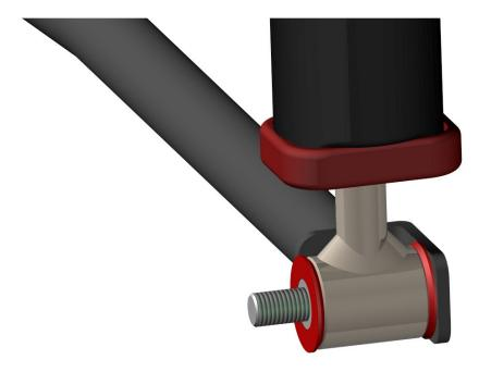
3. Pull the gear linkage pivot out of the gear-stick:
