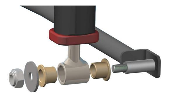
8. Tighten up using the **new** nylock nut:
